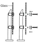
6. Adjusting the height and gap for the whole glass. Use the spanner to fasten the screw.
